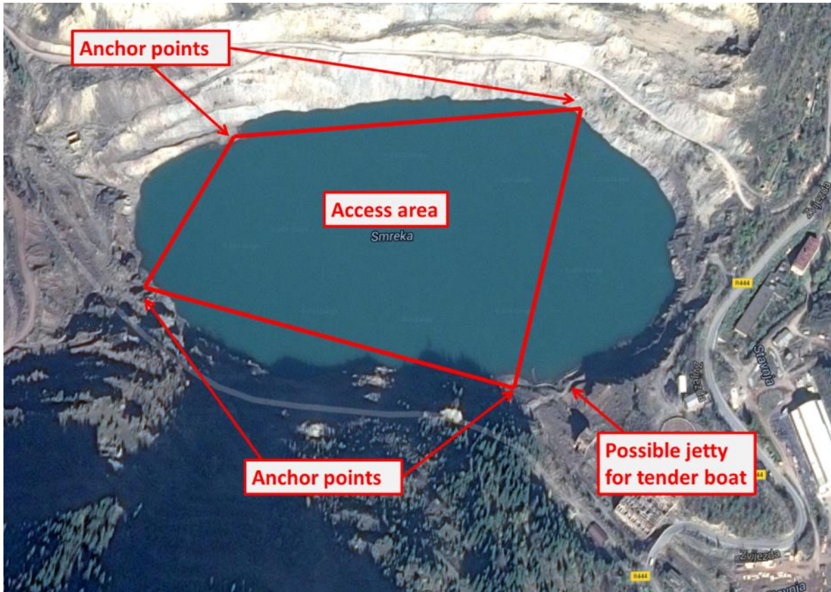
Figure 24 - Plan view showing possible location of anchors for vessel manoeuvring
